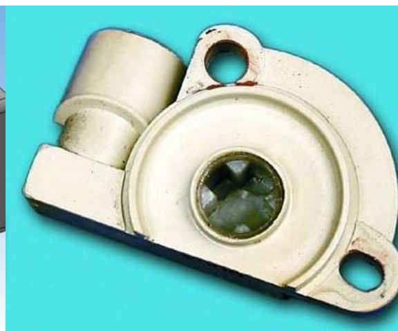
Fig. 4. The sensor of gearshift lever displacement (position) (model 36.3855)
