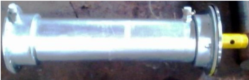
Fig. 2. Working sample of a hydraulic cylinder with a self-releasing screw pair for rotation of the working body
