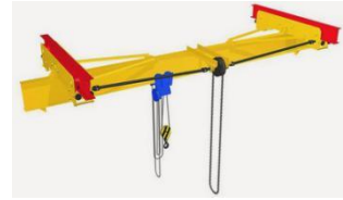
Fig. 5. Manually operated bridge crane
