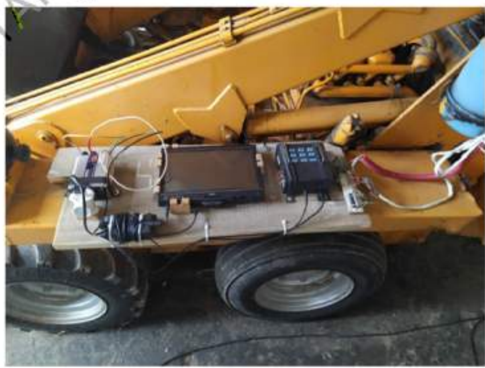
Figure 3 – Information measuring system installed on a small-sized front loader
