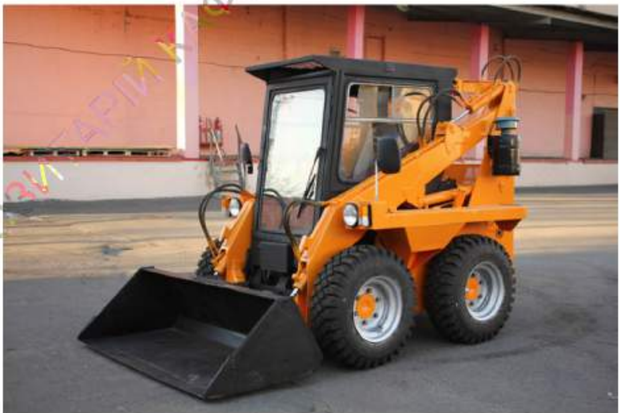
Figure 1 – A small-sized front-mounted single-bucket loader UNC-060
