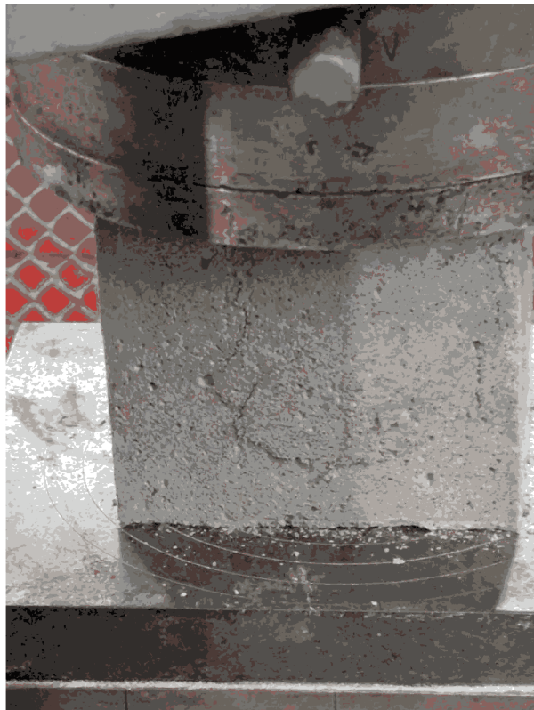
Fig. 2 - Destruction of aerated concrete sample
