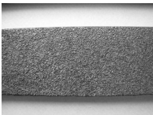
Figure 4 – The appearance of the sample surface, hardened by steel 15H11MFSH
