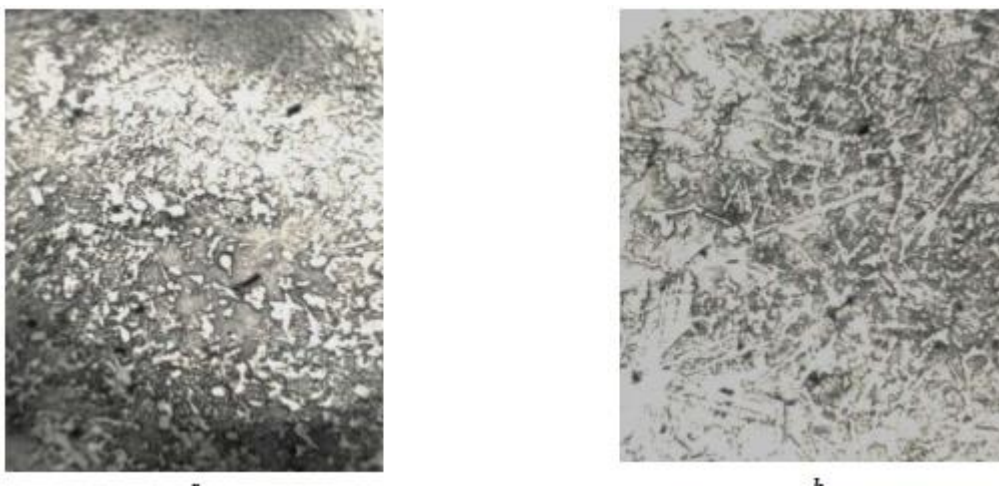
Fig. 2. Structure of powders for spraying PG-SR4 coatings
